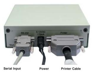
Figure 110: P2RS Parallel-to-Serial Converter Connection Cables
