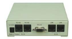
Figure 139: TCPIP 232 Adapter Rear Panel
